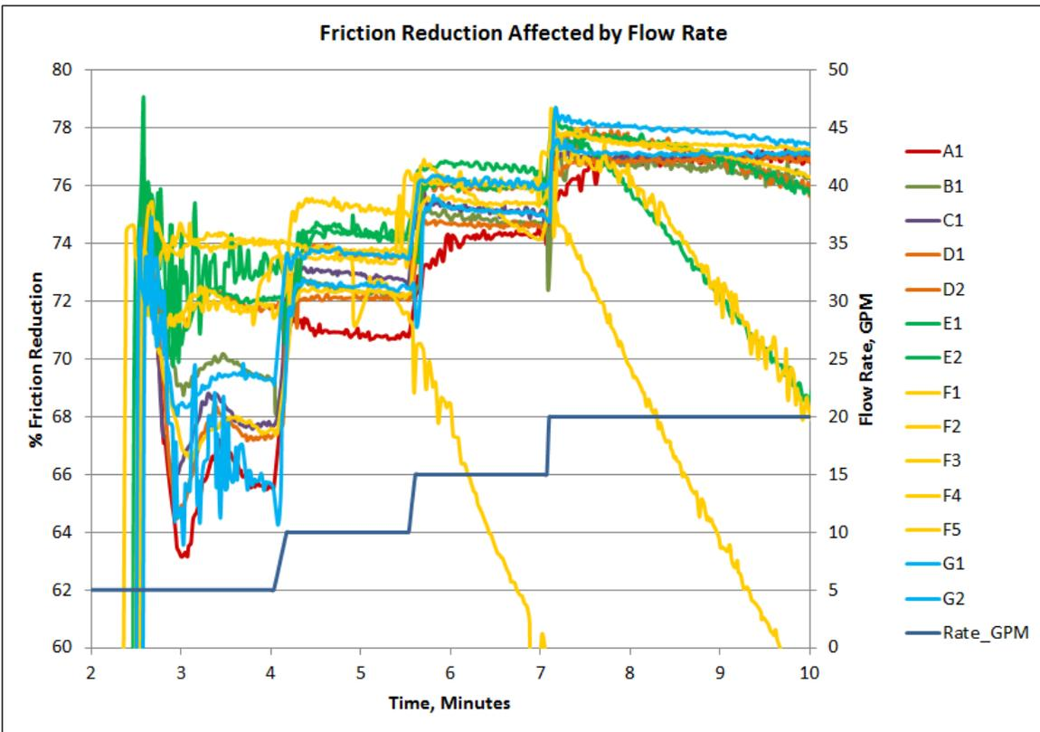
Figure 13 Friction Reduction Results with Varied Flow Rates
