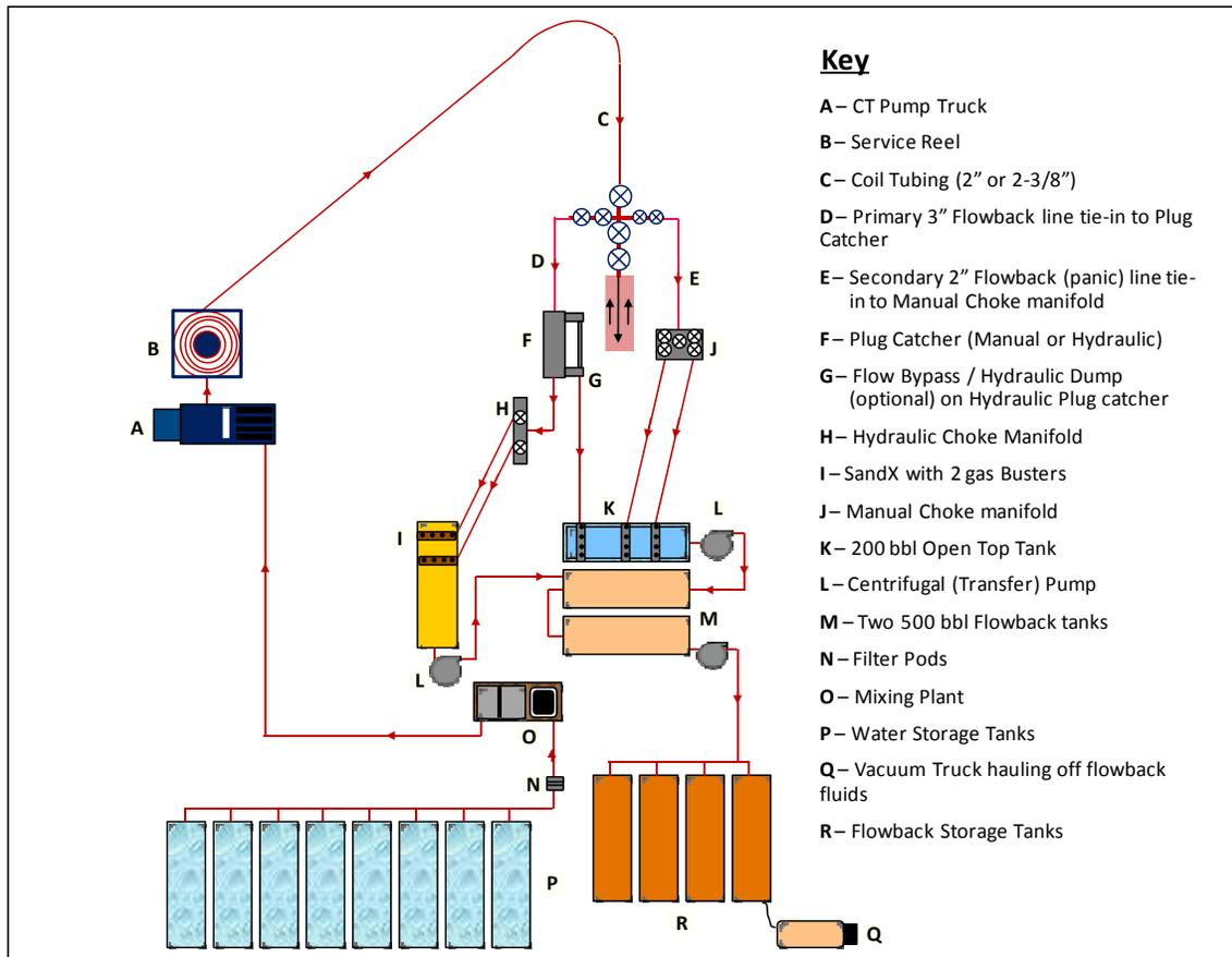
Figure 4 Single Pass Fluid Flow Loop
