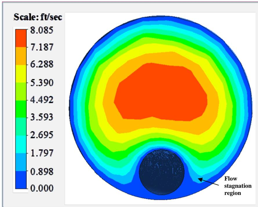
Figure 2 Typical Axial Flow Velocity Profile in Eccentric Annulus (Asafa and Shah, 2012)
