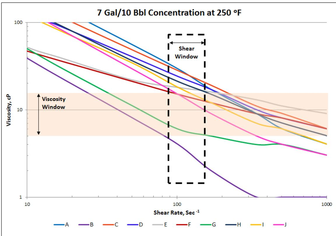
Figure 11 Gel Sweep Viscosity at 7 Gal/10 Bbl and 250°F
