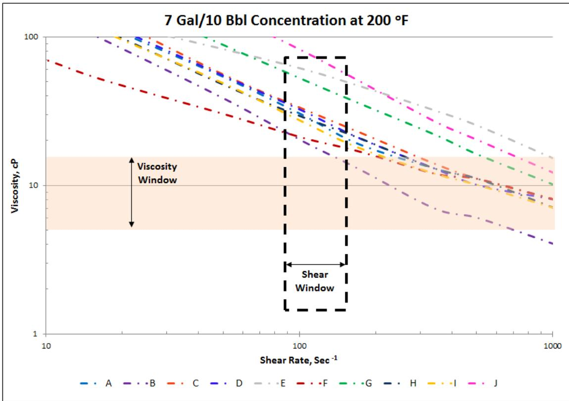
Figure 10 Gel Sweep Viscosity at 7 Gal/10 Bbl and 200°F
