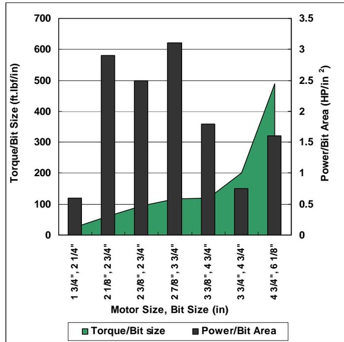
Figure 5 Drilling Motor vs. MTSI & Torque Per Bit Size (Portman and Short, 2000)
