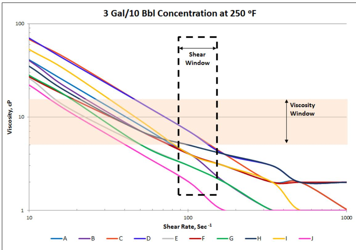
Figure 7 Gel Sweep Viscosity at 3 Gal/10 Bbl and 250°F
