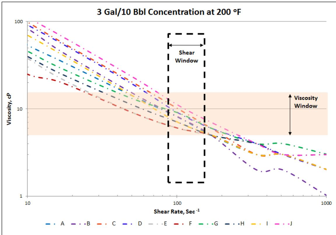
Figure 6 Gel Sweep Viscosity at 3 Gal/10 bbl and 200°F
