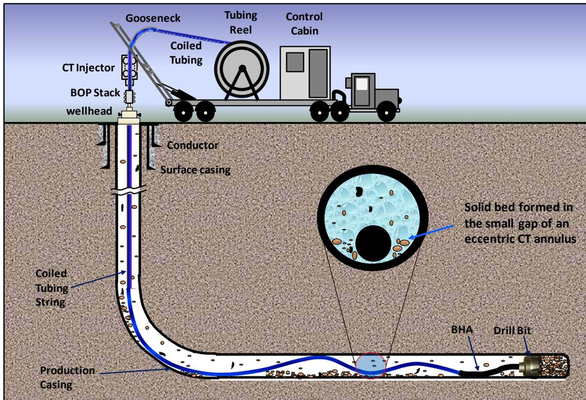
Figure 1 Slurry Flow in Coiled tubing Annulus
