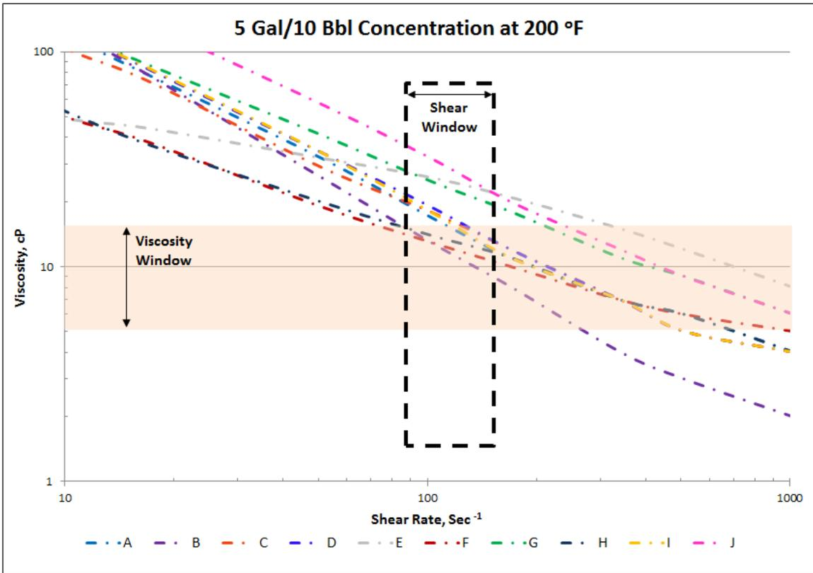
Figure 8 Gel Sweep Viscosity at 5 Gal/10 Bbl and 200°F
