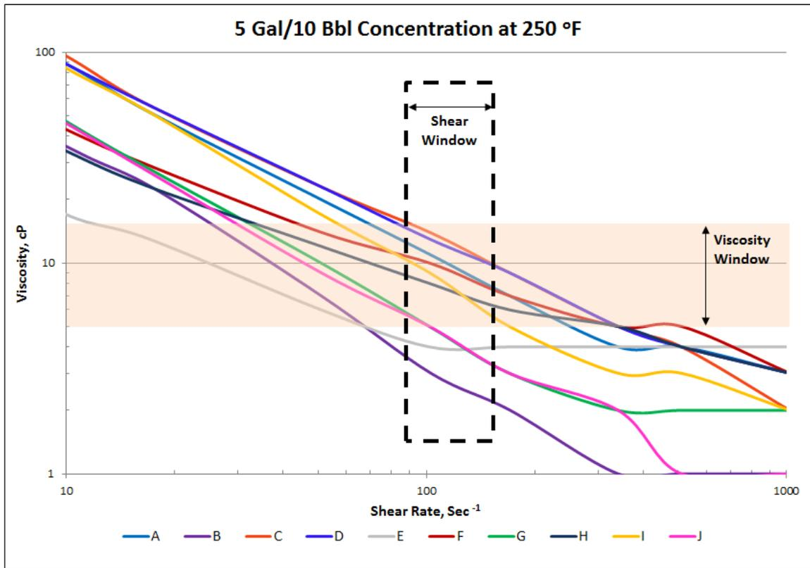
Figure 9 Gel Sweep Viscosity at 5 Gal/10 Bbl and 250°F
