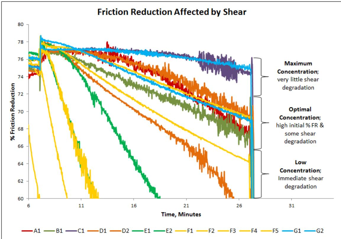
Figure 14 Friction Reduction Results with High Rate and Shear
