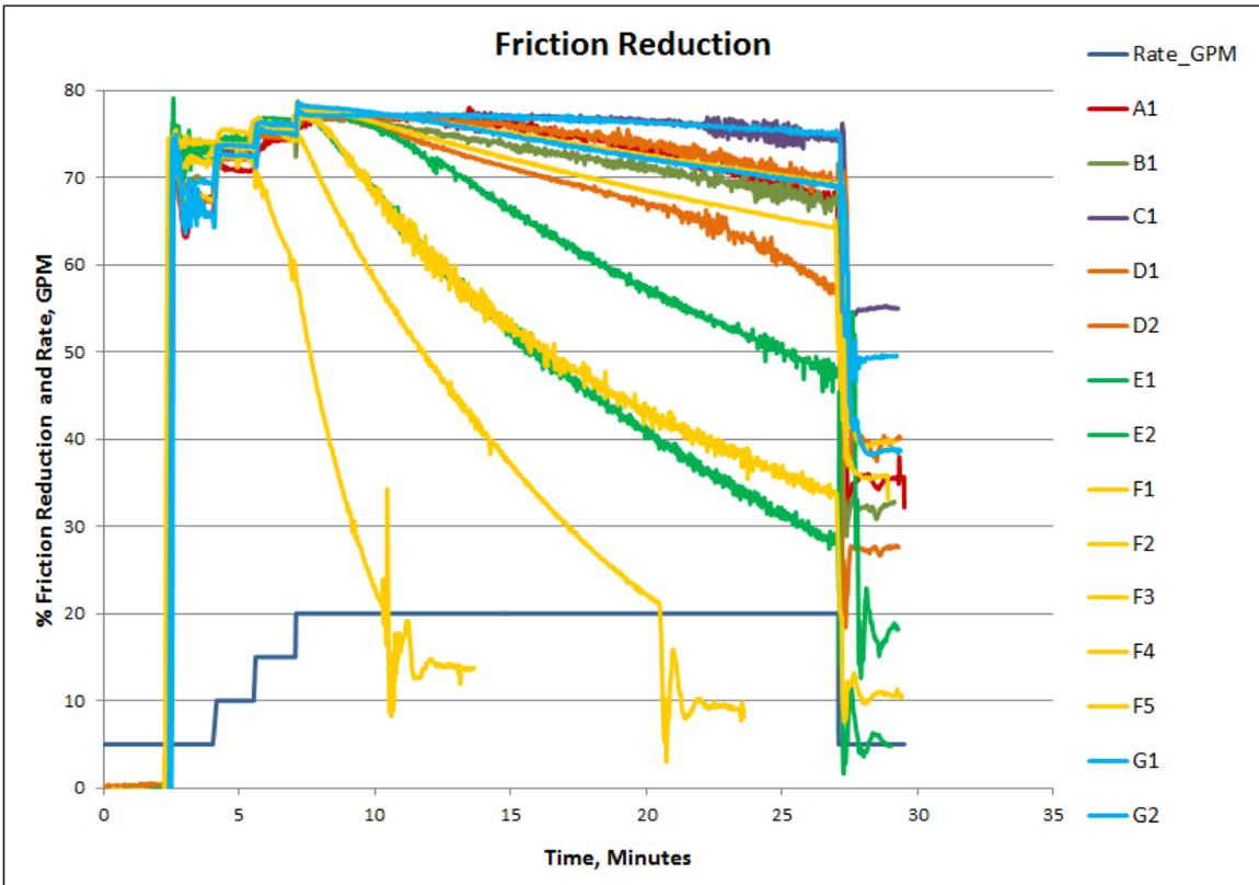
Figure 12 Percent Friction Reduction for All Samples and Concentrations
