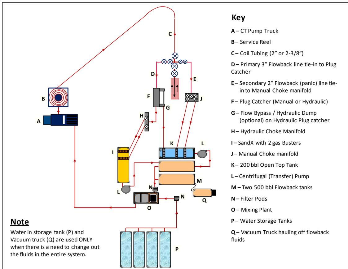
Figure 3 Re-Circulated Fluid Flow Loop
